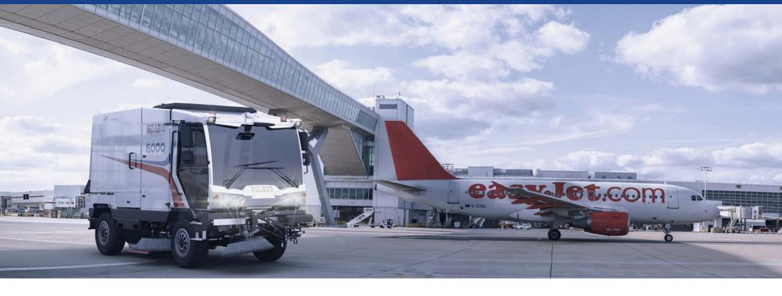
**D**umping Height – USA standards, for the American market, Dulevo designed a specific optional in order to accomplish US standards for street sweepers. Dumping height can vary from 45.3 inches to up to 118.2 inches, facilitating therefore the unload of the collected debris in a high-capacity container.
