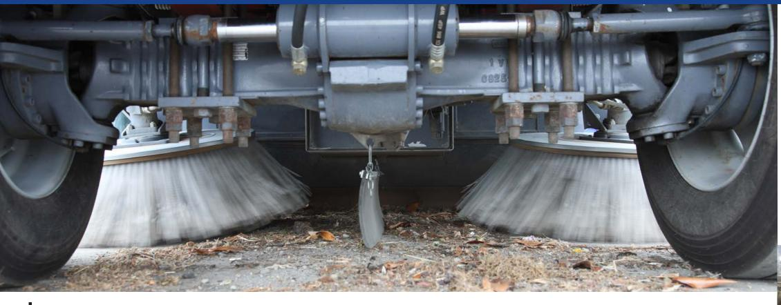
In cooperation with Gore® Dulevo developed the only worldwide existing full fine dust filtration sweeper. This mechanical-suction filtration system grants with the exclusive application of the Gore® technology a total abatement of PM10 particles.
