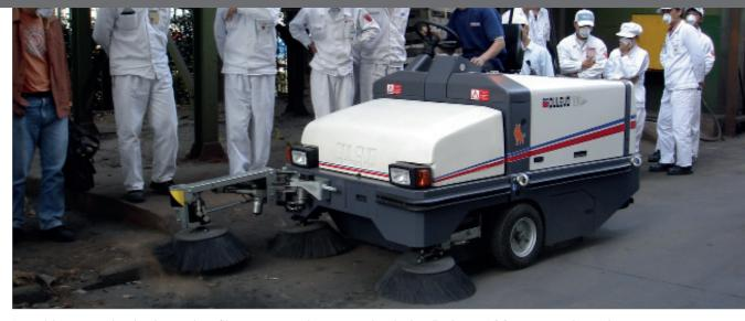
In addition to the high quality filter mounted as standard, the Dulevo 100 man on board sweeper can also be equipped with an even higher performance filter. Gore® technology guarantees the best filtering results thanks to: improved dust control (up to 1 micron), improved aspiration, easier and more economical maintenance.
