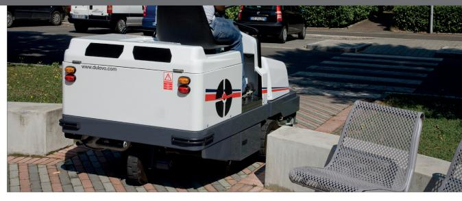
In addition to the high quality filter mounted as standard, the Dulevo 1300 man on board sweeper can also be equipped with an even higher performance filter. Gore® technology guarantees the best filtering results thanks to: improved dust control (up to 1 micron), improved aspiration, easier and more economical maintenance.
