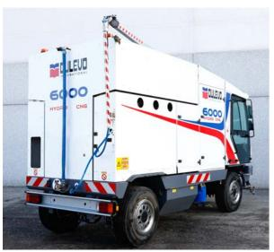
The machine can be configured, according to the customer's needs, with high pressure systems and automatic dosing systems for the sanitizing product.
