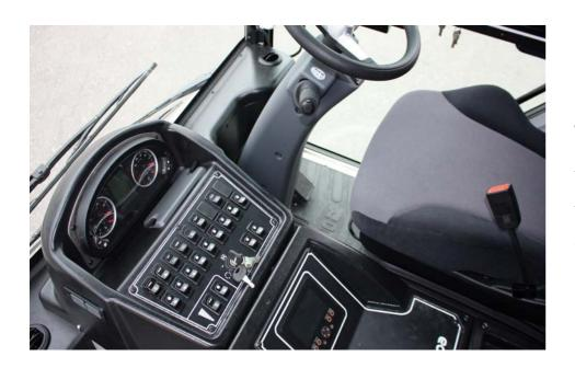
The cabin has been designed so as to guarantee the maximum comfort for the operator and the easiest use. Comfortable, soundproof and with large glass surfaces, the cockpit of these two models of street washers makes work pleasant in any kind of condition. The hydrostatic driving, the power steering and just few controls make the vehicle easy and pleasant to use.
