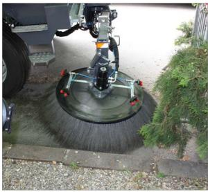
The 180-degree full motion massive front brush is an indispensable auxiliary tool for sweeping corners, gutters and for increasing working width.
