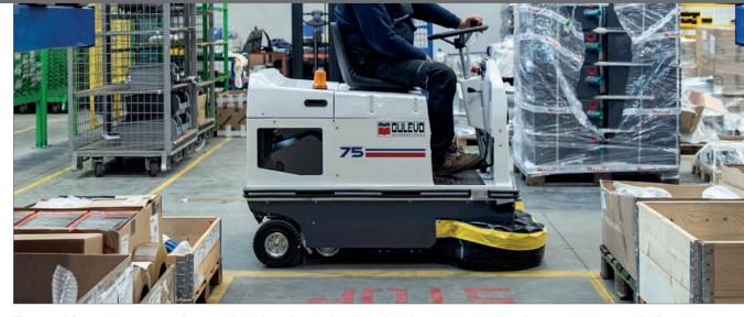
To simplify maintenance, the machine has been designed with easy access to the power unit and all major components. The waste container, which can be removed laterally, is characterized by its large capacity and easy handling ensured by 4 sliding wheels and a comfortable towing handle.
