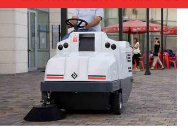
The Dulevo 1100 and 1300 are sweepers that offer the best results in the field of industrial and indoor cleaning. Thanks to their ultra-compact design and hydraulic mechanisms, they are extremely maneuverable, easy and pleasant to drive The total absence of drive belts on the motor components make these ultra-compact all-hydraulic sweepers practically indestructible, helping to significantly reduce routine maintenance costs.
