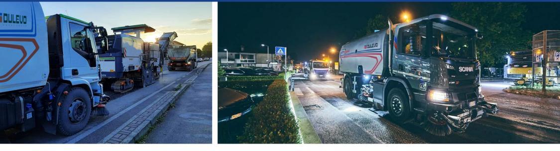
The high suction capacity is guaranteed by the independent auxiliary engine with low polluting emissions: great power and maximum respect for the environment. A mechanical transmission connects the motor and the fan, and allows for always constant suction performance, even in intense use. A proven system that guarantees maximum reliability and extreme simplicity of maintenance in favour of high operating performance and minimum operating costs.
