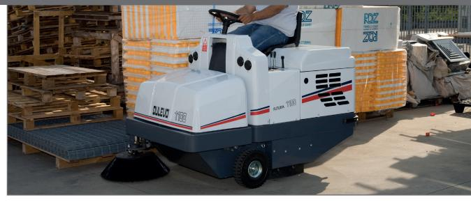
In addition to the high quality filter mounted as standard, the Dulevo 1100 man on board sweeper can also be equipped with an even higher performance filter. Gore® technology guarantees the best filtering results thanks to: improved dust control (up to 1 micron), improved aspiration, easier and more economical maintenance.
