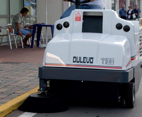
Easy access to all components and entirely hydraulic technology render the sweeper simple and cheap. The 1100 sweeper is available in the BS version with a petrol and LPG engine, DL diesel version, suitable for outdoor areas, and the EH version with battery-powered engine, for indoor and outdoor areas. Each version can also be enriched with an extensive range of accessories.
