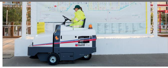
In addition to the high quality filter mounted as standard, the Dulevo 90 man on board sweeper can also be equipped with an even higher performance filter. Gore® technology guarantees the best filtering results thanks to: improved dust control (up to 1 micron), improved aspiration, easier and more economical maintenance.
